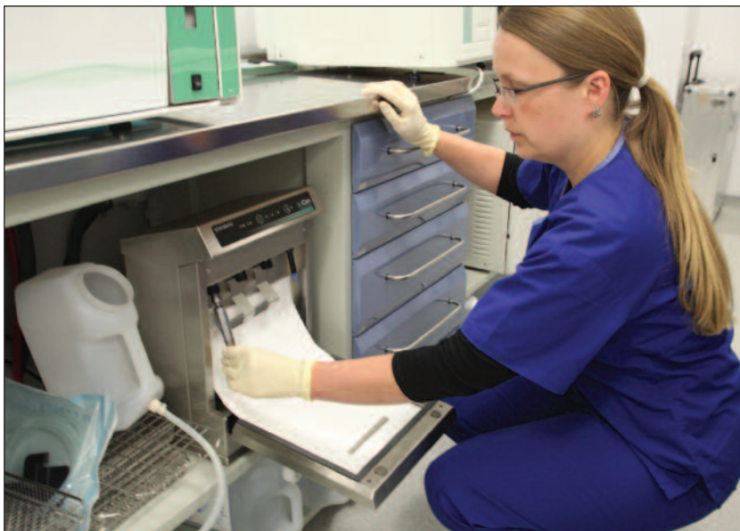
Figure 4: Lubrication of handpieces using the Statmatic handpiece processing centre
