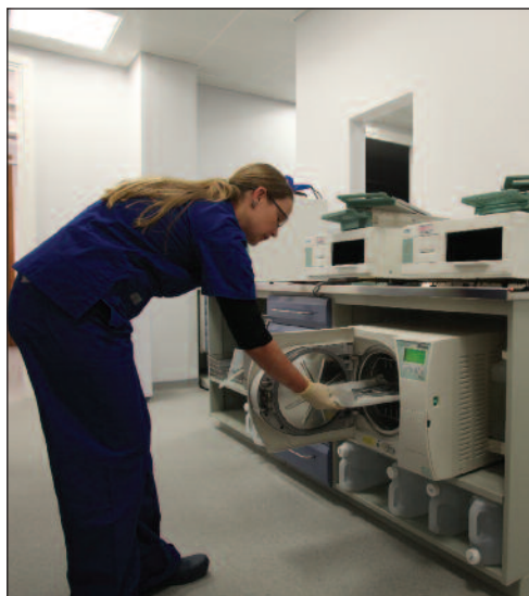
Figure 6: Larger trays are processed in the Bravo vacuum autoclave
