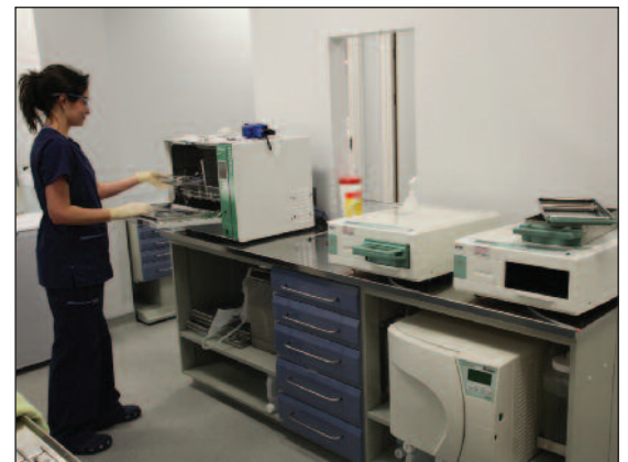
Figure 3: Loading of instruments into the Hydrim washer/disinfector, using the supplied baskets for ease of transfer
