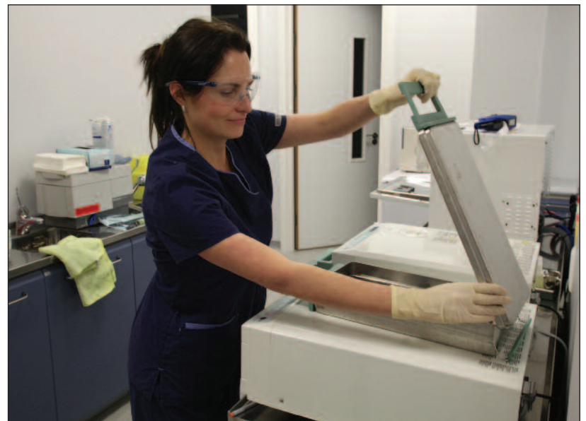
Figure 5: Easy transfer of instruments from the Hydrim washer-disinfector to the Statim autoclave using the baskets
